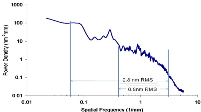
Power spectrum of a surface roughness trace. The RMS is just the square root of the area under the power spectrum. So the RMS increases with longer scale lengths, and decreases with shorter ones.
