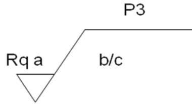
Where a = the RMS roughness specification
