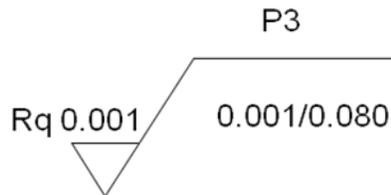
Alternatively, one can simply add a spatial period range to the roughness note, such as “RMS roughness shall be less than 1nm for scale lengths from 1 micron to 80 microns.” That, at least, will result in a meaningful specification.
