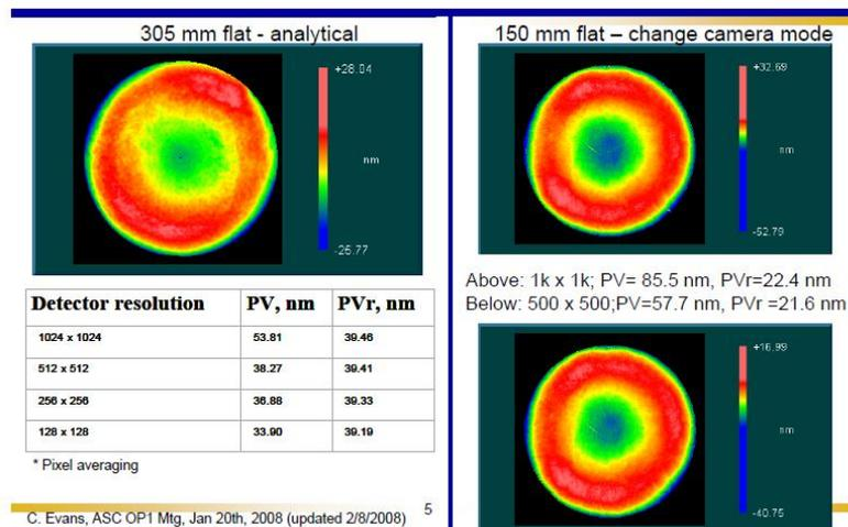
*Figure from ASC/OP meeting minutes, showing the stability of PVr compared to PV for various interferometer resolutions*
